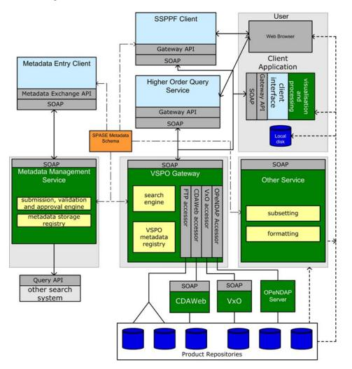
Fig. 3. VS3O system architecture diagram showing extended capability for the VSPO system.
