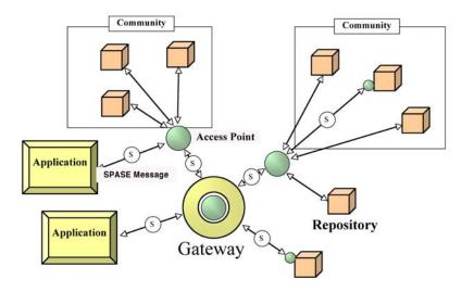
**Fig. 1**. A possible data environment architecture. Information and data flows from repositories to applications through access points and gateways. The portions of the system using SPASE-Data-Model-based messages are indicated with the S.
